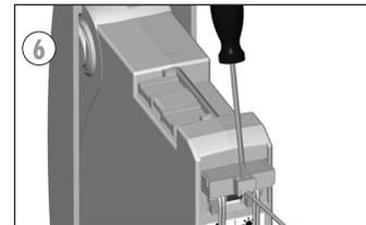
**Example:** Dismantling a flush-mounted belt winder.
