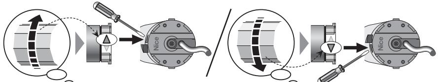
04. Use the wall-mounted pushbutton strip to adjust the other limit switch so that the rolling shutter (or awning) is at the desired level for this limit switch.
