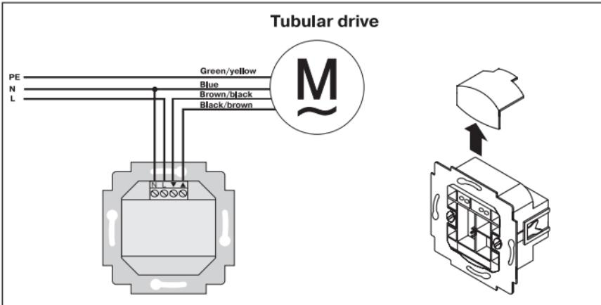
2. Put the protective caps back on the power supply unit.
