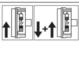
Switch the radio switch to the inside position. If the radio switch is already in this position, switch it to the outside and back to the inside position.
